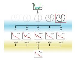
Recent advances in Wide-angled X-ray Scattering techniques (WAXS) offer the ability to probe transient changes in protein conformations down to picosecond levels, [1] and at resolutions down to secondary structure levels where their fluctuations become apparent. [2] These information can be translated into constraints on conformational averages which are complementary to distance-based constraints such as NMR, and will assist in the characterisation of large-macromolecular complexes.
